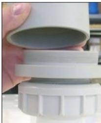
2. Remove the filter casing.
