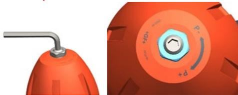
4. Set the concentrate pressure to 1 bar  $\pm$  0.2 by turning the concentrate valve (emergency operation valve) (26). The pressure can - read 0-4 bar on the manometer.
