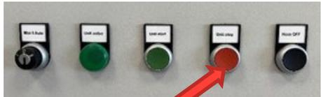
Press the red button to stop the device. The green light will turn off.
