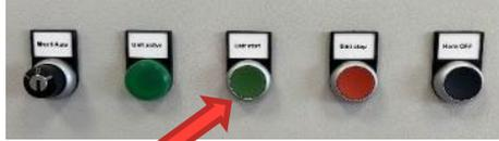
Press the green button to start the device. The green light will turn on.
