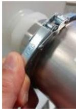
1. Remove the safety pin and open the clip.
