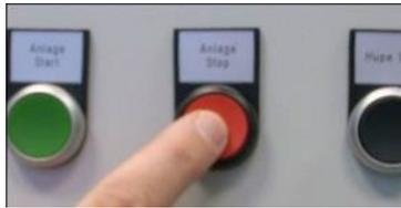
At any time, Hot Cleaning can be stopped by pressing the red button. The unit cools down independently.
