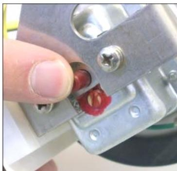
3. Re-activate the safety fuse by pressing on the red safety button
