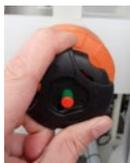
10. Reopen the membrane valve. Ensure that the filter is not leaking.
