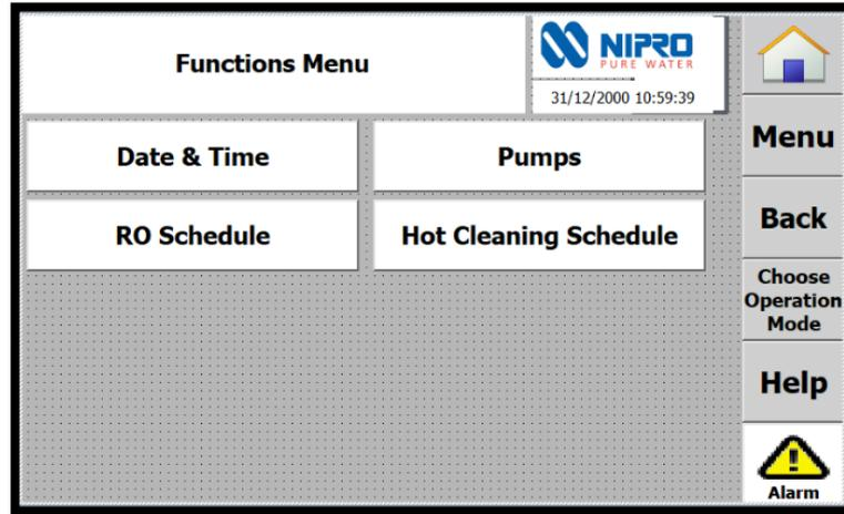
In this menu, two start and stop timers can be set per day. Select the day the RO system should start and enter the start time and stop time.
