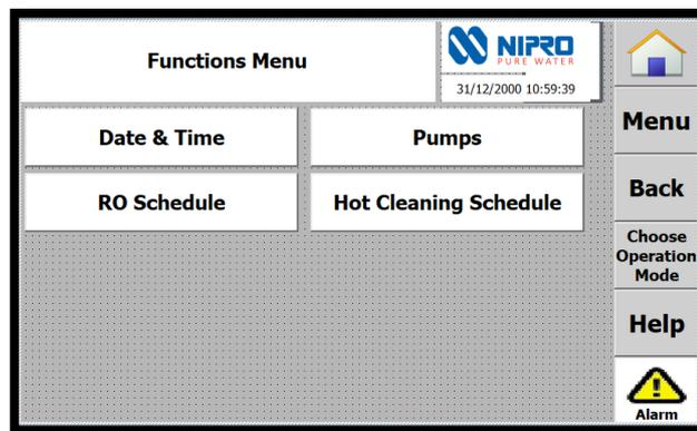
Select the weekday when Hot Cleaning is needed. For Phoenix One DS+, a preheating option is available. This option allows the hot water tank to be filled and pre-heated during normal operation and the Hot Cleaning starts at the set time.
