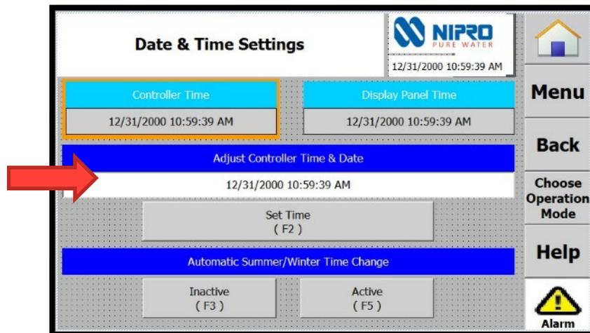
Tap on **Set Time** or press the **F2** button on the display panel to confirm the new settings:
