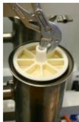
6. Pull the membrane out by using a tong.
