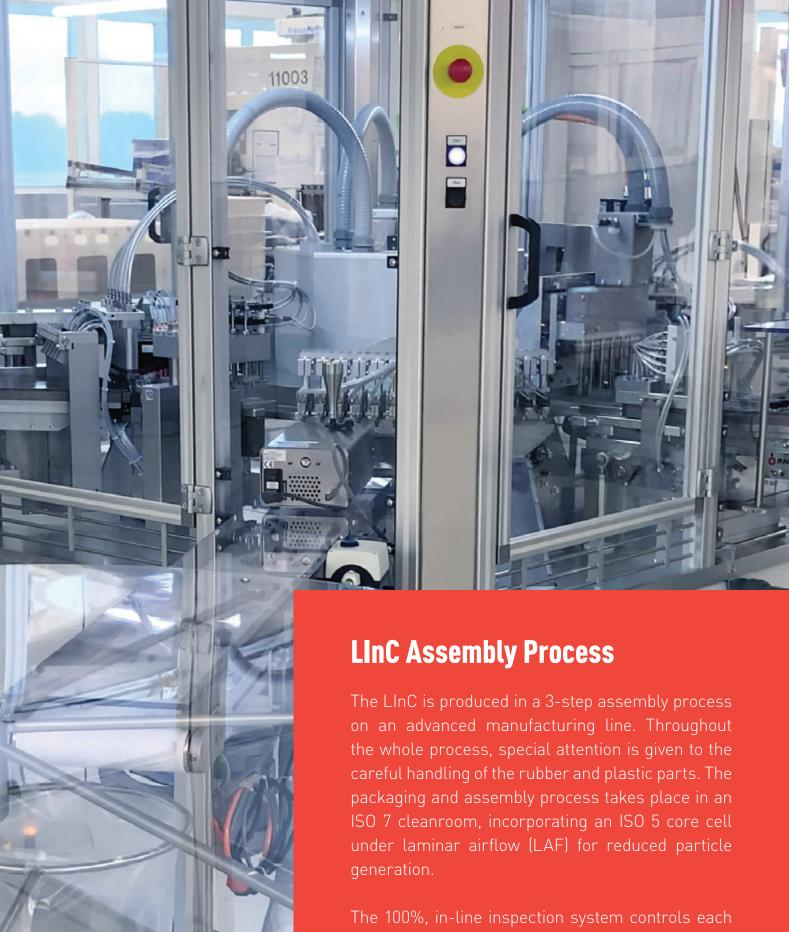
The 100%, in-line inspection system controls each LInC for various quality aspects. Statistical process control (SPC) further ensures that all products comply to agreed quality specifications.
